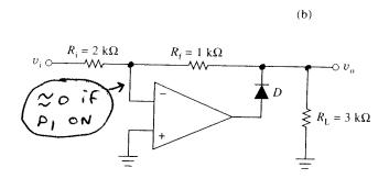
If Vi > 0, then D1 is OFF, and the OP AMP is disconnected from the circuit
