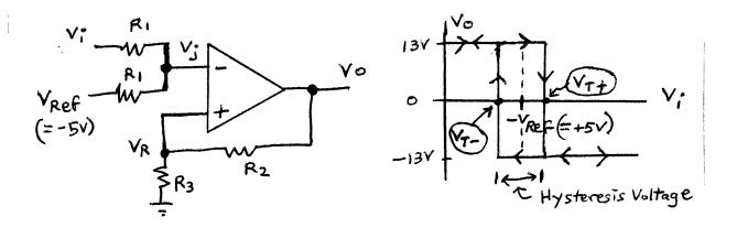
By linear superposition, the voltage at the (-) input of the op amp, Vj, is
