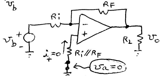
The  $R_i//R_F$  resistance may be replaced by a short circuit, since there is no voltage dropped across  $R_i//R_F$ , since  $i_+ = 0$  (Rule #2 of OP AMP). Thus we have the "inverting OP AMP configuration"
