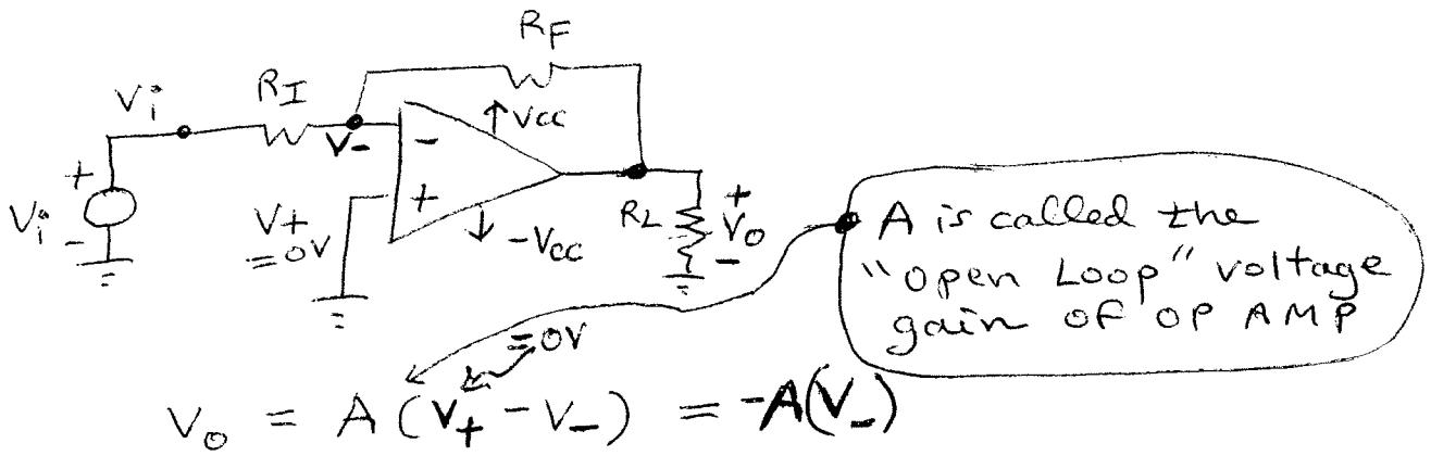
Since no current flows into (-) input of OP AMP, by linear superposition we see
