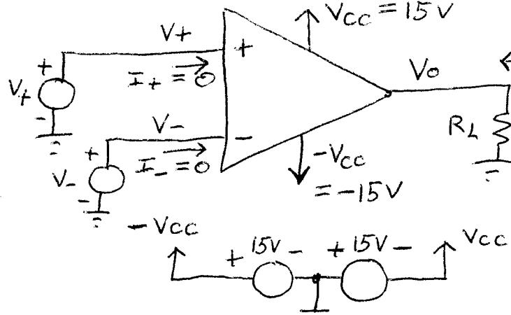
"Typical" Op Amps have protective current limiting circuitry that limits  $I_o$  to:
