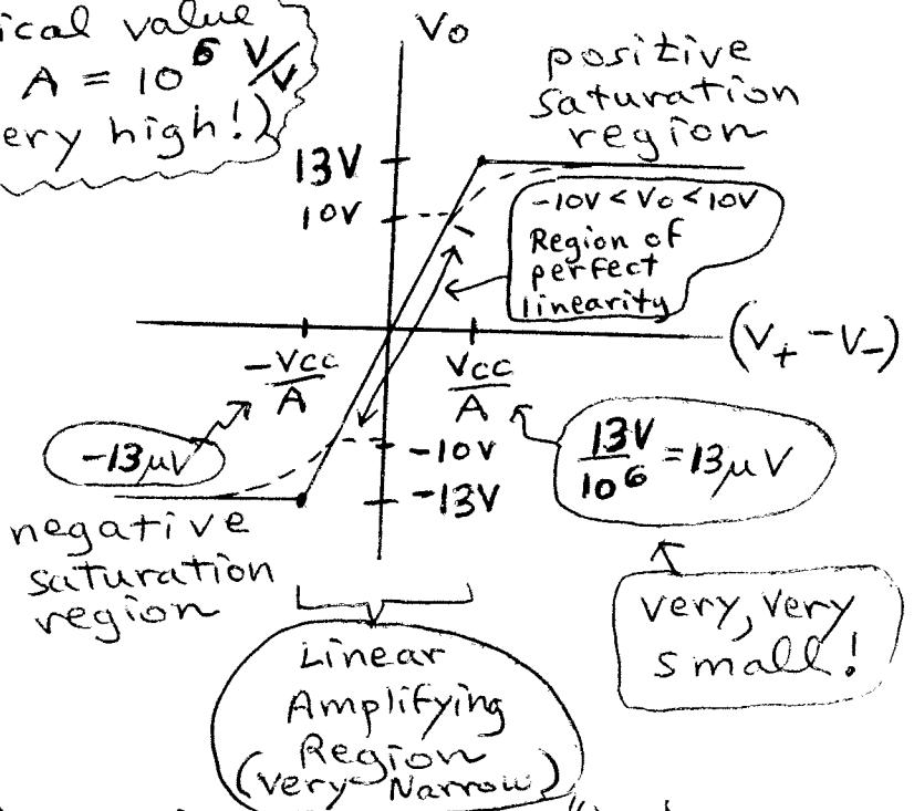
Rule #1 of OPAMP: ("Virtual Voltage Rule") When OP AMP is operating in its linear amplifying range,  $V_+ \approx V_-$ , since  $(V_+ - V_-)$  must lie between  $+15\mu\text{V}$  and  $-15\mu\text{V}$ .
