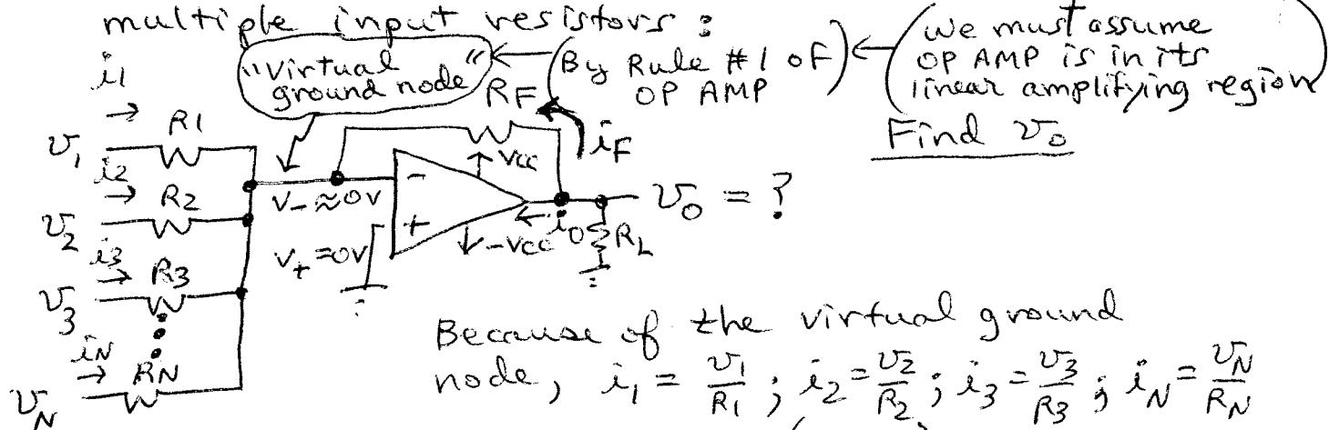
Because of the virtual ground node,  $i_1 = \frac{v_1}{R_1}; i_2 = \frac{v_2}{R_2}; i_3 = \frac{v_3}{R_3}; \dots; i_N = \frac{v_N}{R_N}$
