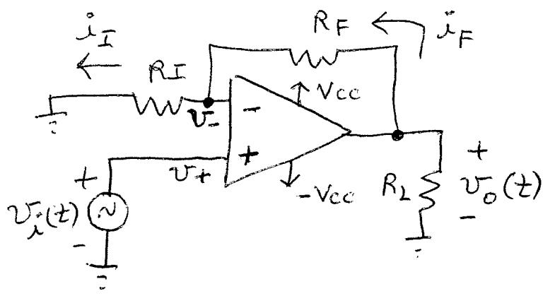
Find the closed-loop voltage gain  $A_v \triangleq \frac{v_o}{v_i}$
