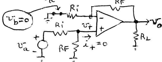
Because  $i_+ = 0$ , we may use a voltage divider eqn to find  $v_+$ , then from  $v_+$  to  $v_o$ , we have a "non-inverting OP AMP config."
