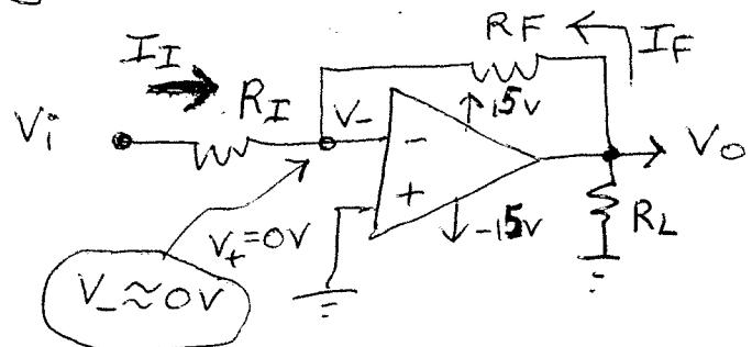
By Rule #1 (Virtual Voltage Rule)  $V_-$  is "virtually at ground" since  $V_+ \approx$  at ground.
