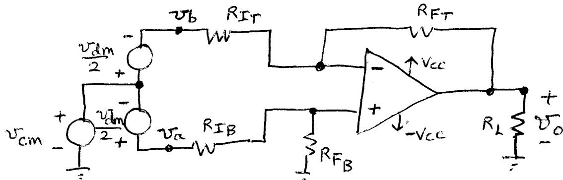
Also note that the  $R_f$  &  $R_I$  resistors have been differentiated using the subscripts T (top) and B (bottom).
