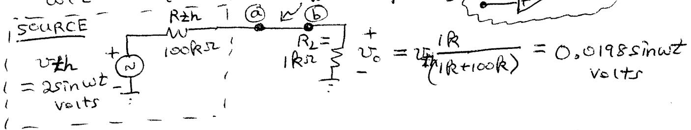
with the op amp voltage follower removed, far less signal gets delivered to the load due to the presence of the  $100k\Omega$  resistor. We say that the op amp follower circuit eliminates the effects of "Loading" a source with a high Thevenin resistance when it is connected across a relatively low load resistance " $R_L$ ".
