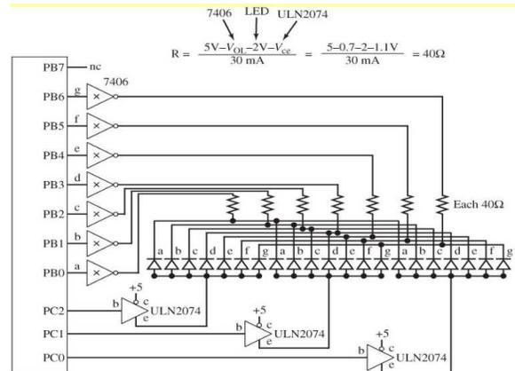
For MC9S12C32, replace PB with PT and PC with PM.
