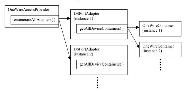
Figure 6 shows the common features of a 'container'. A device that contains memory will create a 'memory bank' instance for each memory bank. The memory is divided up into banks depending on the feature set of the bank. For example one bank could be volatile while another is nonvolatile. Or a bank could be general-purpose memory or it could be 'memory-mapped' to change the functionality of the device.
