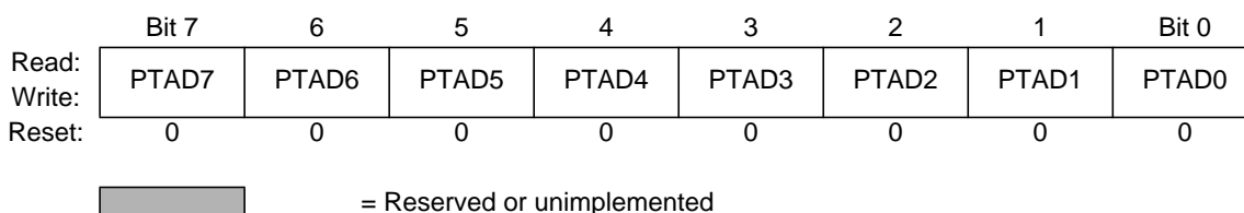
Figure 3-38 Port AD I/O Register (PTAD)
