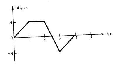
4) (a) Plot the "g" wave from Problem 3 as a function of distance at the fixed time t = 2 s. Remember this wave is traveling in the -z direction with a velocity magnitude of 300 m/s. (Partial answer: your plot should show that g(2s,300m) = -A)
