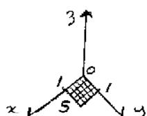
$$\begin{aligned} \vec{B} &= 3xy^2 \vec{i}_z & d\vec{s} &= dx dy \vec{i}_z \\ \vec{B} \cdot d\vec{s} &= (3xy^2 \vec{i}_z) \cdot (dx dy \vec{i}_z) = 3xy^2 dx dy \\ [\Phi]_S &= \int_S \vec{B} \cdot d\vec{s} = \int_S \int_{x=0}^1 \int_{y=0}^1 3xy^2 dx dy \end{aligned}$$
