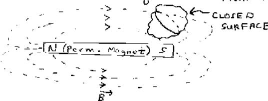
We see that the field's set up by magnetic objects (dipoles) (like permanent or electro-magnets) having both North & South poles will always obey this rule - no matter where the closed surface is placed. If we could find a magnetic "monopole", say, an object, that originates flux but does not "receive it" again, we could place this
