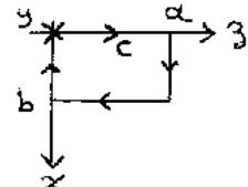
$$[\text{EMF induced}] = - \frac{d}{dt} [\phi]_{\text{into paper}} = ab B_0 \omega \sin \omega t$$
