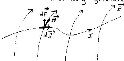
Ampere's Law of Force predicts that the incremental force,  $d\vec{F}$ , exerted on an incremental segment of wire,  $d\vec{l}$ , is given by
