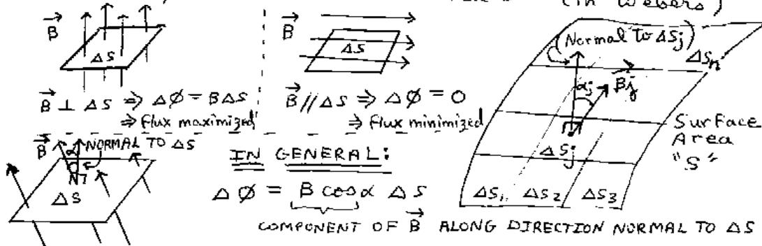
The net magnetic flux crossing the surface  $S$  must therefore be given (approximately) by:
