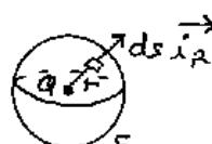
Then, if we choose a (Gaussian) surface that is a sphere of radius  $r$ , over which  $D$  is uniform, and then apply Gauss' Law over this surface,
