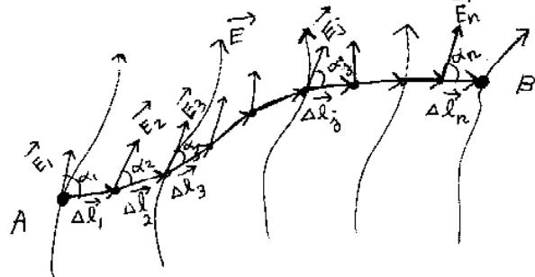
The voltage or Electromotive force (EMF) at  $B$  w.r.t.  $A$  is the work done in carrying a 1-coulomb charge from point  $A$  to point  $B$ :
