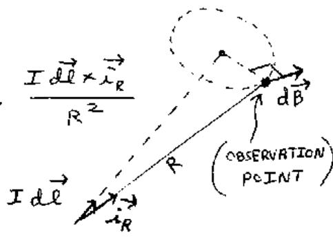
Therefore the force on a current-carrying wire segment  $I_1 dl_1$  in the presence of the magnetic flux density  $d\vec{B}$  produced by a current-carrying wire segment  $I dl$  is given by:
