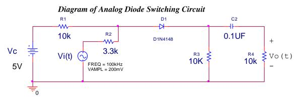
Build this circuit using a 1N4148 small-signal diode. Set your dc power supply to deliver +5 Vdc, and use this for the control voltage "Vc" in Fig. 1-18 on p. 1.51 of the Class Notes. Also, set up your function generator to deliver a 200 mV (peak-peak) sine wave at a frequency of 100 kHz. Let  $C = 0.1 \mu$ F. Note that the magnitude of the impedance of this value of C at the specified source frequency (100 kHz) is
