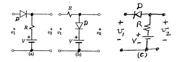
Partial answers for Part (B): Circuit (a) : While v1 < 4.7 V => v2 = 4 V (D off); while v1 > 4.7 V, v2 = v1 - 0.7 V (D on) Circuit (b): While v1 < 4.7 V, v2 = v1 (D off); while v1 > 4.7 V, v2 = 4.7 V (D on) Circuit (c): While v1 < 3.3 V, v2 = v1 + 0.7 V (D on); while v1 > 3.3 V, v2 = 4 V (D off)
