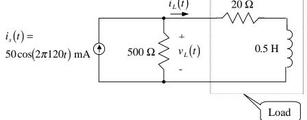
54. The circuit shown below is in the sinusoidal steady state.
