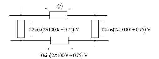
10. Use phasors to find the voltage  $\underline{V}$  in the circuit mesh shown below. Then express your answer as a time function v(t). Draw a phasor diagram showing your calculation.
