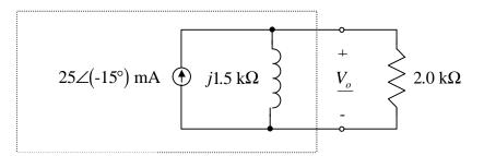
40. In the circuit shown below, replace the nonideal source by its Norton equivalent. Then use the current divider to find  $I_o$ .
