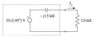
41. Use series and parallel combinations, voltage and current dividers, and source transformations as appropriate to find  $V_o$  in the circuit shown below.
