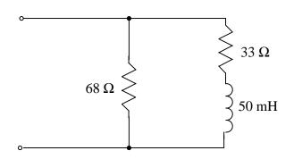
28. Find the equivalent impedance of the combination of elements shown below at a frequency of 40 MHz.
