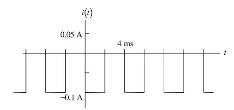
49. Find the effective (RMS) value of the voltage waveform shown below.
