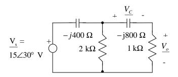
37. Use the voltage divider to find the phasor  $V_c$ . Plot  $V_c$  to scale on a phasor diagram for  $\omega = 1$ , 10, 100, and 500 r/s.
