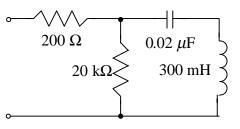
30. Find the equivalent impedance of the combination of elements shown below at a frequency of
