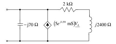
32. Find  $\underline{V_C}$  and  $\underline{I_L}$ . Plot  $\underline{I_s}$ ,  $\underline{V_C}$ , and  $\underline{I_L}$  on a phasor diagram.
