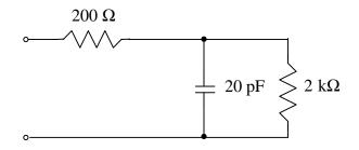
29. Find the equivalent impedance of the combination of elements shown below at a frequency of 12,000 rad/s.
