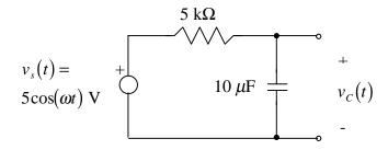
38. The circuit below is in the sinusoidal steady state. Use the current divider to find  $I_c$ . Then find  $i_c(t)$ .
