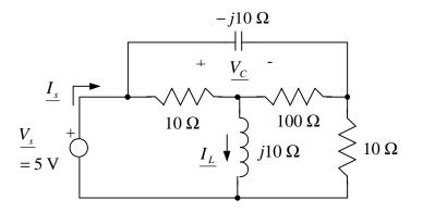
36. Find  $\underline{V_c}$  and  $\underline{V_o}$ . Plot  $\underline{V_s}$ ,  $\underline{V_c}$  and  $\underline{V_o}$  to scale on a phasor diagram.
