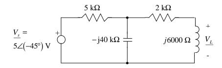
35. Find  $\underline{I_s}$ ,  $\underline{V_c}$ , and  $\underline{I_L}$ . Plot  $\underline{V_s}$  and  $\underline{V_c}$  to scale on a phasor diagram. Plot  $\underline{I_s}$  and  $\underline{I_L}$  to scale on a second phasor diagram.
