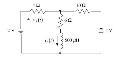
14. The circuit shown below contains one constant source and one source that turns *off* at t = 0.
