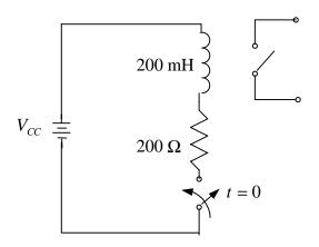
Find  $V_{cc}$  so that the relay will close at t = 2 ms.
