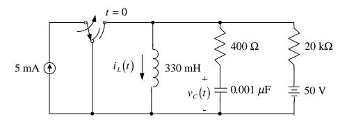
32. In the circuit shown below the switch has been in the lower position for a long time, when it is suddenly moved to the upper position at t = 0.
