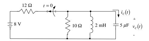
26. In the circuit shown below the switch has been in the position shown for a long time. At t = 0 the switch is suddenly opened.
