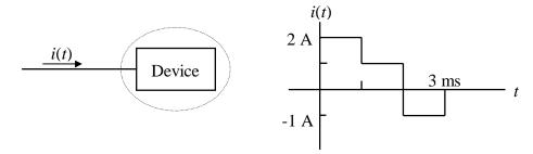
Suppose that the charge stored in the device is zero at time zero. Find and plot the stored charge as a function of time.
