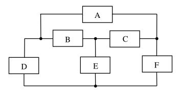
6. In the circuit shown below the current i(t) is given by  $i(t) = 2\cos(2\pi 1000t)$  mA.
