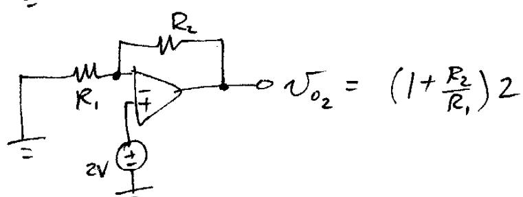
$$V_o = V_{o3} + V_{o2} = -\frac{R_2}{R_1} 3 + 2 + \frac{R_2}{R_1} 2$$
