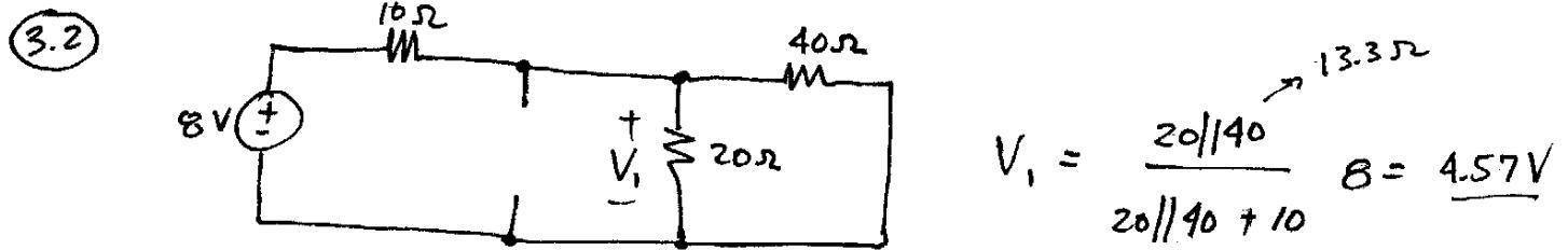
$$V_1 = \frac{20/40}{20/40 + 10} \rightarrow 13.3\Omega \quad B = \underline{4.57V}$$
