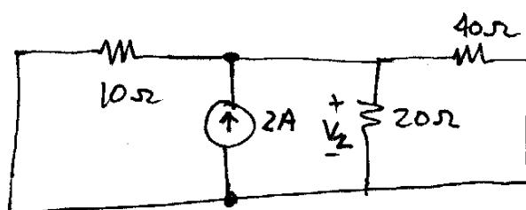
$$\begin{aligned} V_2 &= 2(10||20||40) \\ &= 2(5.71) \\ &= \underline{11.4V} \end{aligned}$$
