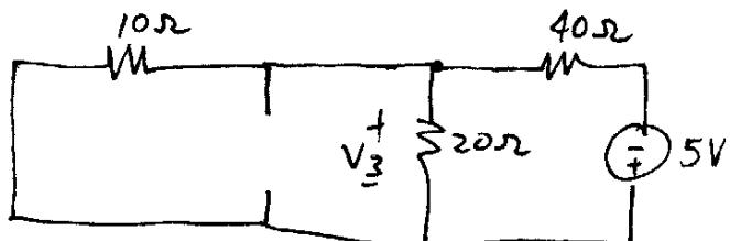
$$\begin{aligned} V_3 &= -\frac{20||10}{20||10 + 40} \rightarrow 6.67V \\ &= \underline{-0.714V} \end{aligned}$$
