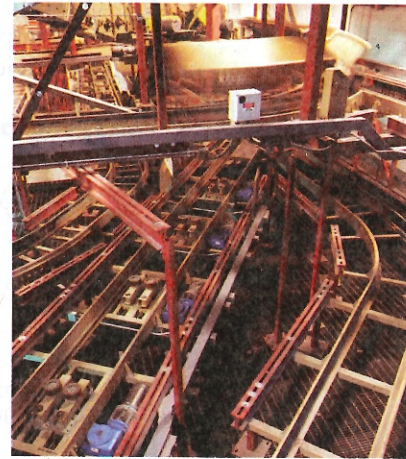
The Denver airport originally had a fully automatic system for moving luggage, replacing human operators with robotic carts. Unfortunately, the system never worked and was dismantled before the airport was opened.
