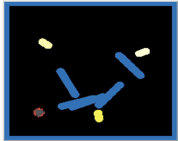
Fig. 1. A typical instantiation of the subCULTron exploration system modelled in Netlogo is shown in the figure. The array of grey circular dots represent the group of connected aMussels (bottom left corner), the red arrows represent the aFish (surrounding the group of aMussels). The long blue patches represent obstacles and the smaller patches in different shades of yellow represent the interesting areas coloured according to how interesting the areas are.
