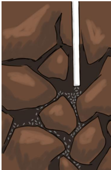
Figure 2: The carbon dioxide is transported down a pipeline and stored in a geological formation. The liquid carbon dioxide fills in the gaps in the porous rocks and over time will turn into chalk, a stable form of carbon dioxide.
