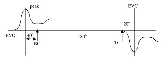
Select an appropriate runner length at the following RPM. Assume the speed of sound in the exhaust gas is 2200 ft/s
