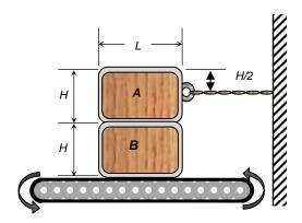
For parts a) and b) assume the two crates stick together and the conveyor belt continuously slips underneath crate B.
