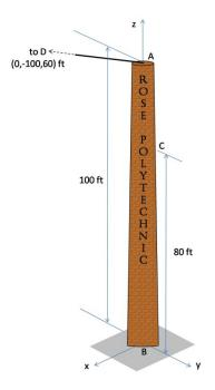
The correct equation of equilibrium for the forces acting on the smoke stack is
