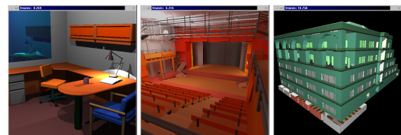
Figure 1: Interactive ray tracing: The office, conference and Soda Hall models contain roughly 40k, 680k, and 8 million triangles, respectively. Using our software ray tracing implementation on a single PC (Dual Pentium-III, 800 MHz, 256MB) at a resolution of 512^2 pixels, these scenes render at roughly 3.6, 3.2, and 1.6 frames per second using both processors.
