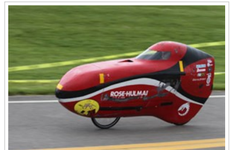
This year's human-powered vehicle incorporated several innovations, including an active aerodynamic wing to counteract crosswind instability.
