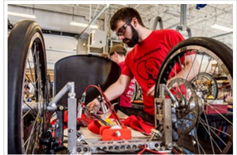
RHEV's redesign of its vehicle, nicknamed "Double Down," included a significantly lighter carbon fiber unibody with aluminum mounting points.
